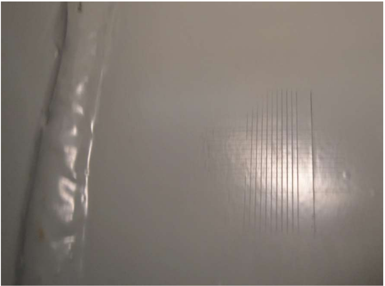
Sample #2 After Boiling Water Cross Hatch Tape Pass
