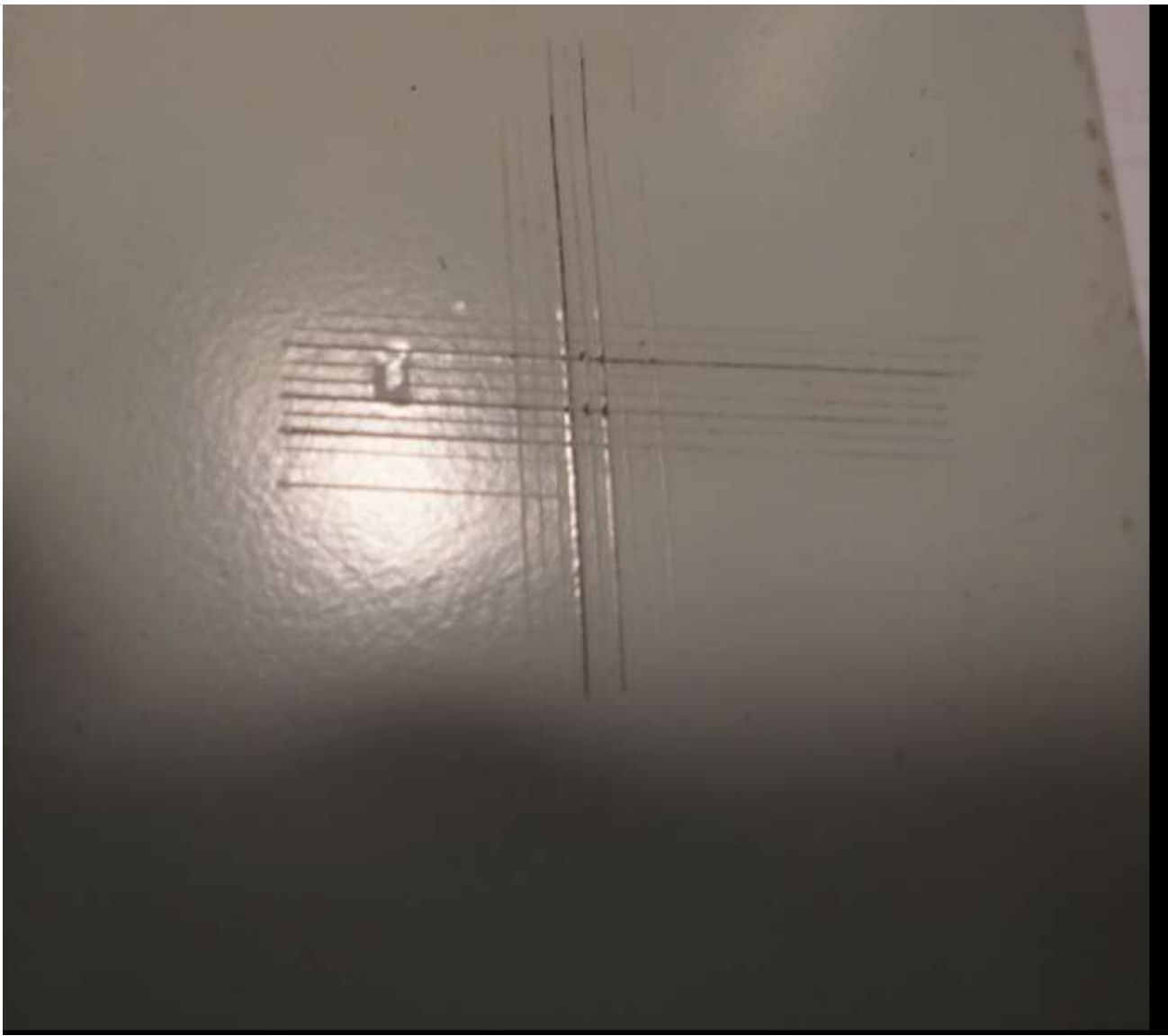
Sample # 3 After Boiling Water Cross Hatch Tape Pass ( Chipping at edge due to blade )
